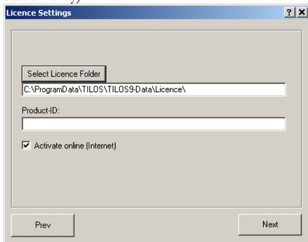
5. Provide the Product-ID and then provide the Serial Number when prompted. Provide the company name and an email address. An internet connection is required to activate the license. The activation is done twice. The second activation will confirm and validate that the License was activated correctly. The license is tied to the computer name, path and MAC address.
