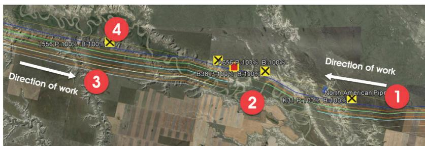
Figure 8. Overlay of TILOS plan and progress in GIS system.
